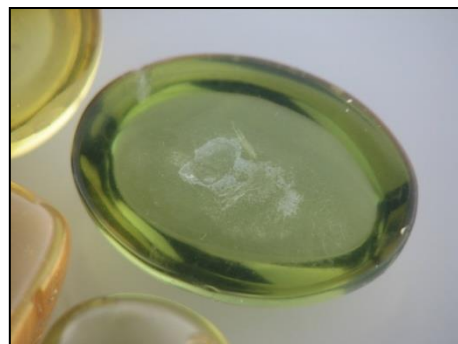
Fig. 4 – Detail of the surface of the “ green amber ” after testing with pure alcohol.
