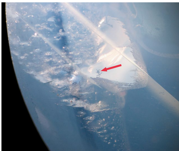
Figure 10: Magnification reveals twin planes and a healing fissure with dotted fluid inclusions in the Roman sapphire intaglio. The larger fluid inclusions show structured expansion discs. The main expansion disc contains tiny, radially arranged needles interpreted as Al-hydroxide precipitates (red arrow). Photomicrograph by M.S. Krzemnicki, SSEF; image width 4 mm.
