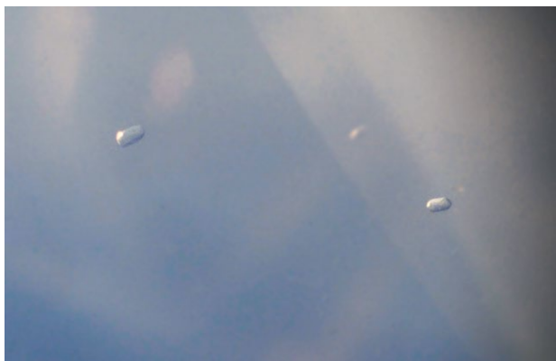
Figure 11: Small idiomorphic plagioclase (albite) inclusions, identified by Raman microspectroscopy, are also present in the sapphire intaglio. Photomicrograph by M. S. Krzemnicki, SSEF; image width 2 mm.
